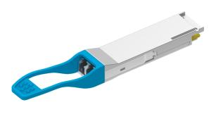
100G QSFP28 LR4 optical Transceiver integrates receiver and transmitter path on one module. In the transmit side, four lanes of serial data streams are recovered, retimed, and passed to four laser drivers. The laser drivers control 4-Distributed Feedback Laser (DFB) with center wavelength of 1296 nm, 1300nm, 1305nm and 1309 nm.
