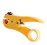
Tool NMC-350 is designed to remove the insulation and trimming with twisted pair. The presence of the wheel for fine adjustment of the depth of the knife moves allows you to make an accurate cut without damaging the insulation of the conductors under the outer shell. A distinctive feature of the NMC-350 is the presence of a spring-loaded cradle for a smooth and uniform course when scrolling around the cable. And the ergonomic design will provide even greater comfort when working.
