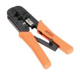
Crimping tools (**Crimper**) are designed for crimping Registered Jack (**RJ**) type connectors on telephone cables and data transmission. **NMC-568R** is designed for crimping RJ45 / 8P8C, RJ12 / 6P6C and RJ11 / 6P4C type connectors. The tool is also equipped with a device for stripping and cutting cables.
