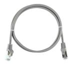
NIKOMAX Essential Patch cords («ES» series) are made from stranded cables, terminated with connectors such as RJ45 /8P8C compliant with T568B standard. Patch cord connectors are protected by boot cover, which significantly increases service life of a patch cord with latch protection.
