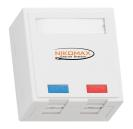
Surface Mount Box are an integral part of horizontal subsystems of SCS and are intended for connection of terminal equipment in workplaces. Structurally, the sockets can be made in two versions: as a complete solution with soldered RJ45 ports and IDC connectors and in the form of a plastic casing into which Keystone plug-in modules are separately installed.
