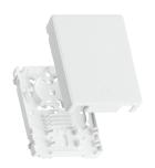
Optical wall sockets are designed to pull the cable out of the wall and connect various terminal equipment to it. It can also be used as a small wall cross. The case of the outlet is made of high quality white. Inside there is a place for laying the cable and two seats for single SC or dual LC adapters. The cable is inserted through a hole in the bottom of the outlet, or one of the connectors.
