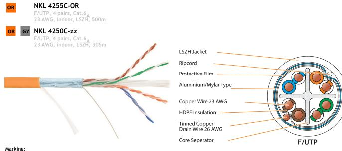
NIKOMAX NETWORK SOLUTIONS /// NIKOLAN NKL 4255C-OR F/UTP SOLID CABLE 4P CATEGORY 6<sub>A</sub> 23AWG Class Dca LSZH (Hr(A)-HFLTx) ISO/IEC 11801 & EN 50173 & ANSI/TIA-568-C.2 NVP 0.69 (ZL) YYMM xxxM
