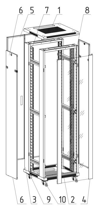
The cabinet is collapsible, with a number of heights 18, 24, 26, 42U and a depth of 600 and 800 mm.
