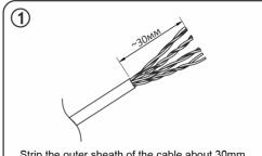
Strip the outer sheath of the cable about 30mm. Remove the breaking thread and cable core separator if present.
